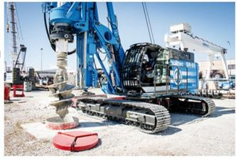
drilling mast; this allows the use of the entire available track for both large diameter tools (working under the lower part of the mast) and long casing segments. The rig can also be equipped with a winch crowd system that can offer a track of more than 16 m with extraction power of 330 kN. The added stroke and power provide the ability to drive longer casing segments in a single pass.
